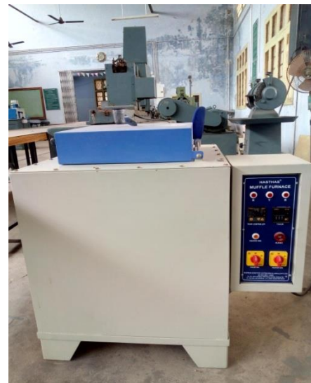
Fig. 2. Preheater electric Furnace
