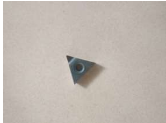
Fig 3. Polycrystalline Cubic Boron Nitride (PCBN) tool
