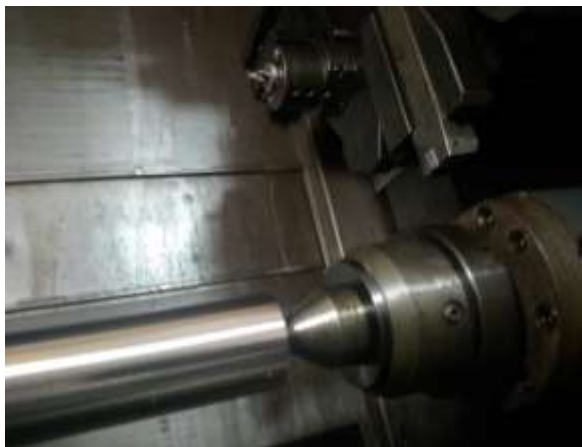
Fig 4 Turning of AISI 4340 alloy steel
