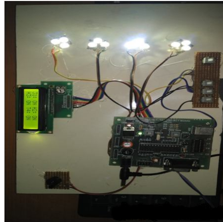
Figure.6.10. Hardware Implementation House hold -1, 2 & 3 Status ON and Theft Identified
