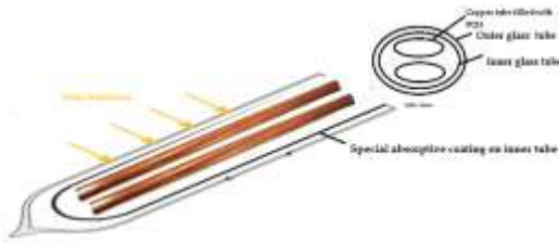
Fig.3.3 Evacuated tube inserted with copper tube
