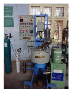
The aluminium alloy LM25 ingots were cut in power hacksaw machine to the small rods of 50 mm thickness and 25 mm diameter to feed the materials in to the crucible. The required proportion of the rods as per experimental plan is fed in to crucible and melted by heating in the induction furnace at the temperature of 725 °C for 1 to 2 hours and melt the rod above its liquidus temperature to make it in the form of semi liquid state (around 600°C).
