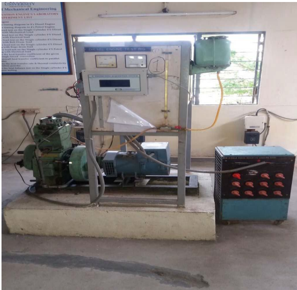
Fig. 5.2 Single cylinder four stroke diesel engine with test rig.
