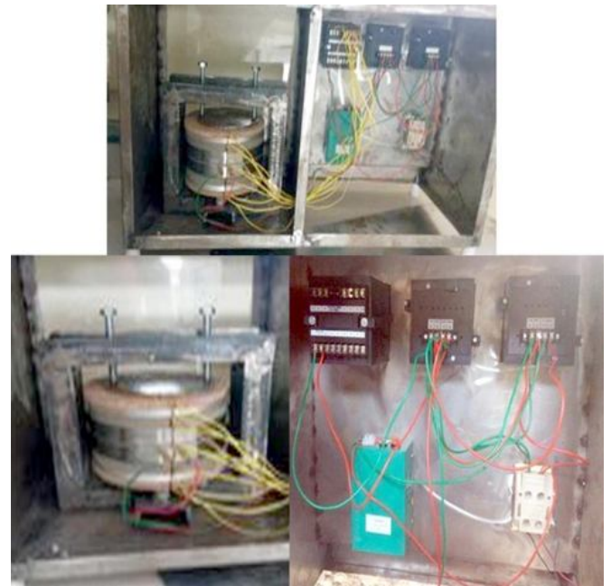
Fig.6.3 Experimental setup of heat flow meter for thermal conductivity test.
