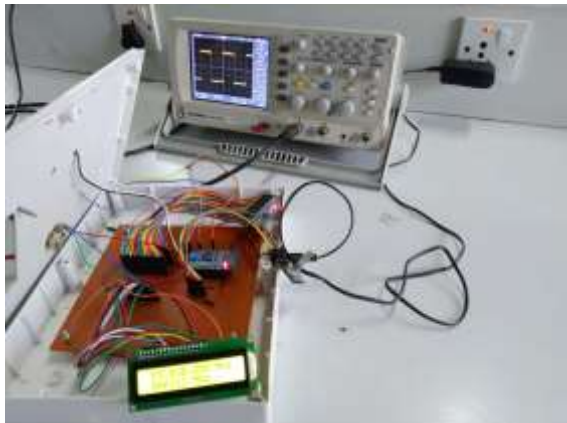
Figure 2 Hardware with square wave output on DSO
