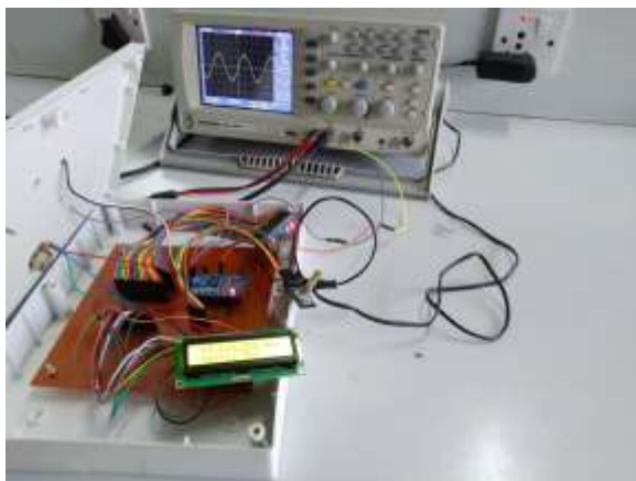
Figure 3 Hardware with sinewave output on DSO
