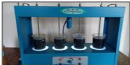
Fig. No. 2: Ink wastewater before coagulation-flocculation on jar test
