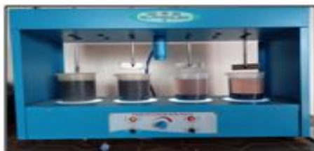
Fig. No. 3: Ink wastewater after coagulation-flocculation on jar test
