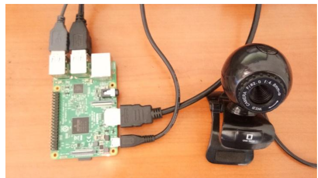
Figure 6 Hardware implementation for emotion detection
