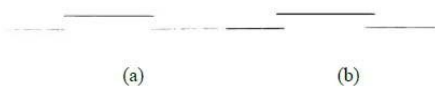
Figure 6. Binary image containing laser blobs (a) before morphological operations are applied and (b) after morphological operations are applied.
