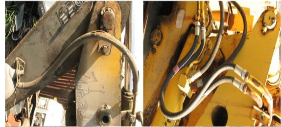
Figure no.1. Example of pressure hoses damaged .[4]
