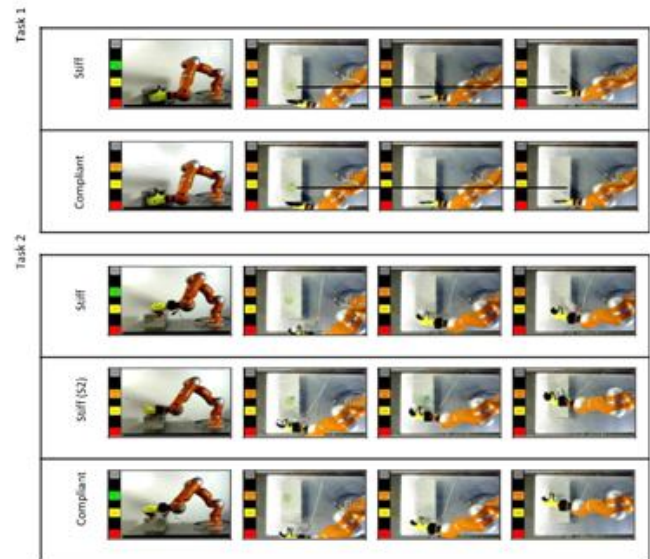
Fig. 5. Screen shots of the heavy object pushing (Task 1) and collision (Task 2) tasks in active mental state (stiff) and neutral mental state (compliant). For the second task, two different examples of the active (stiff) case for the two subjects are provided.
