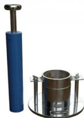
FIG: 19 LIGHT COMPACTION TEST APPARATUS (RAMAR AND MOULD ALONG WITH BASE PLATE)
