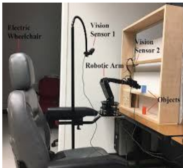
Figure 1. Image of the robotic arm mounted on an electric wheelchair
