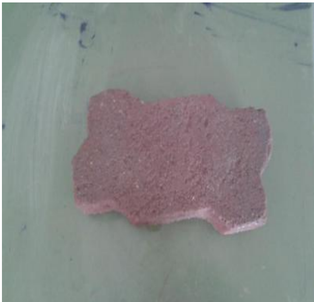
Fig 6: Efflorescence test on plastic sand brick
