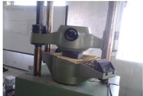
Fig 3: Compressive strength for plastic sand bricks
