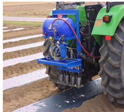
Fig 6. machine frame with electro-pneumatic components
