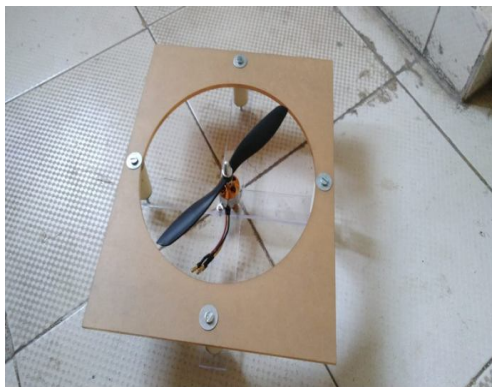
Vacuum fan is used for adhesion of robot on wall.
