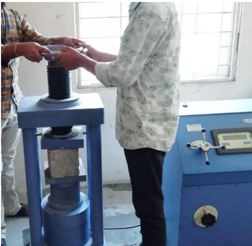
Fig.3.1 compressive strength of cubes
