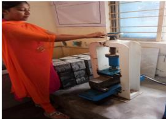
Fig.3.3 Flexural Strength of Cubes
