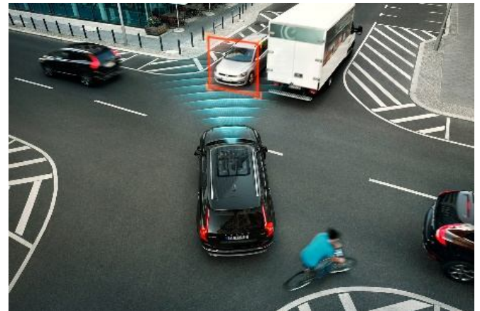
Figure 2: Driverless car sensing the environment
