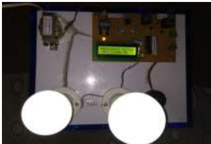
Figure 4:- Both Loads are in ON position during rated supply
