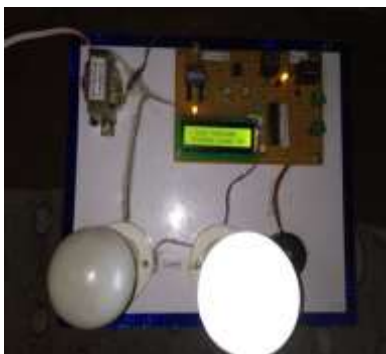
Figure 5:- Primary load is OFF and secondary is ON during under voltage supply
