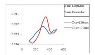
From the result it is found the length of 356 mm and diameter of 178mm shows the optimum pressure, velocity and sound for fire extinguisher.
