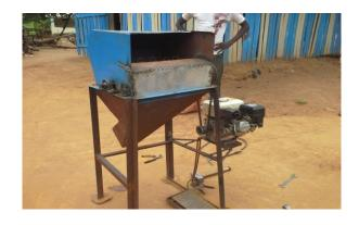
Although they are gradually being replaced by combine-harvesters, motorized threshing- machines still have an important place in the postharvest production process, especially for their convertibility. By the simple replacement of a few accessories and the appropriate changes in settings, these machines can treat different kinds of grain (e.g. rice, maize, sorghum, beans, sunflowers, wheat, soybeans, etc.).
