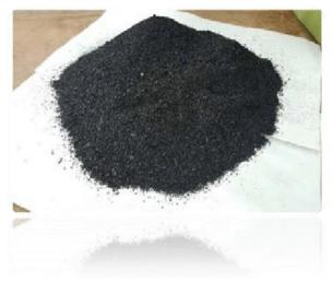
Fig. 2- saw dust ash
