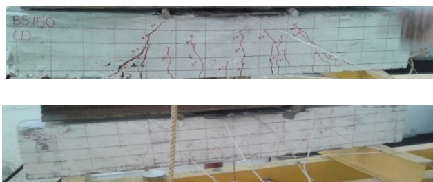
Figure 8: conventional beam & A1 Beam
