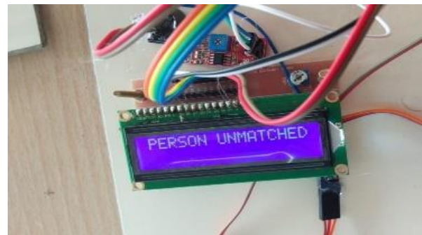
Fig III The above image shows that when unauthorized person comes in front of the door, the camera compares with the stored image and displays that the person is unmatched.
