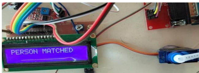
Fig I This shows when the person comes in front of the door, the camera captures the images and the captured image is compared with the stored image. When the images are same, the LCD displays that the person is matched.
