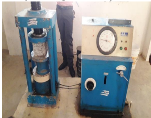
Fig no 1 Compressive Strength Test
