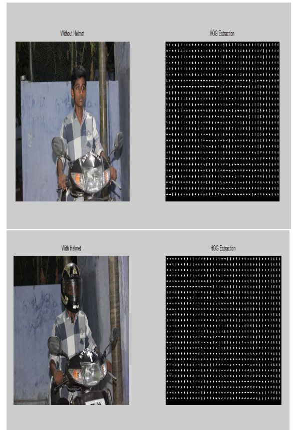
Fig 5.Histogram of Oriented Gradients
