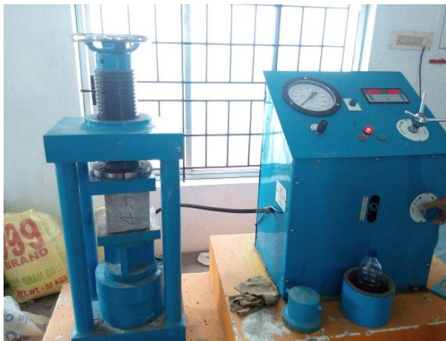
Fig 3 Compression testing of cubes
