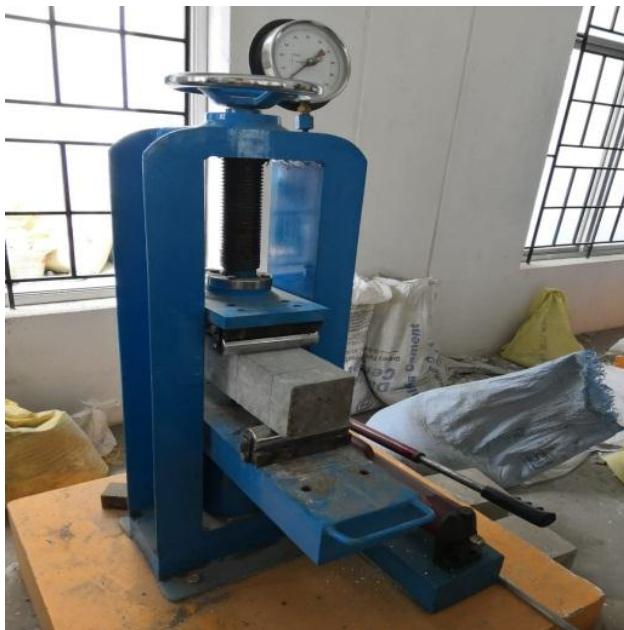
Fig 4 Flexural strength testing of beams
