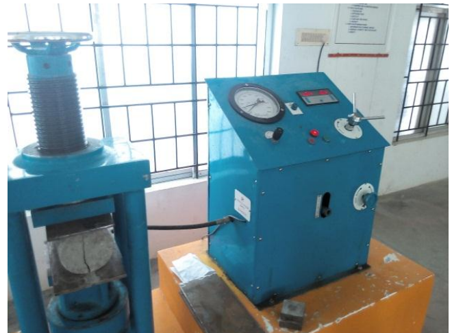
Fig 5 Split Tensile testing of cylinders
