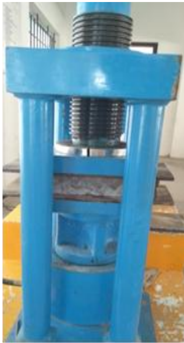
Figure 2: Compression strength test
