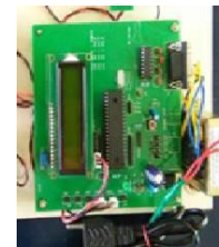
Fig. 6 : (a) AT89s52 Microcontroller assembly set, (b) Speaker section, (c) Receiver section
