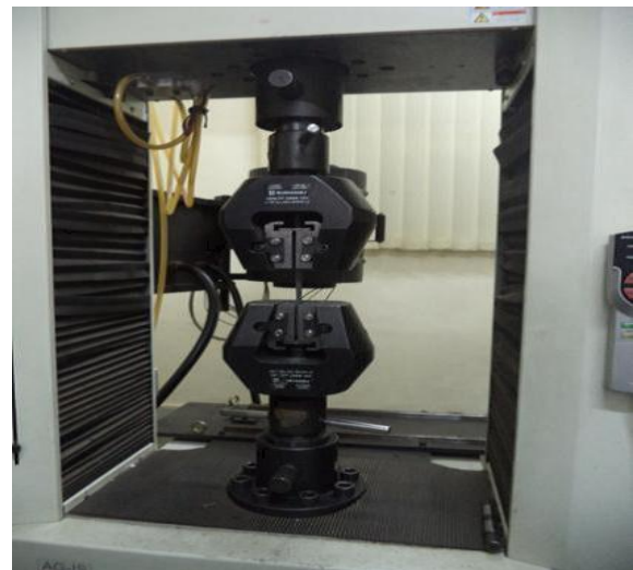
Fig. 4 Specimen subjected to Tension Test on UTM.
