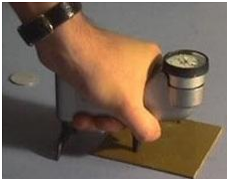
Fig.6 Hardness Test Fixture
