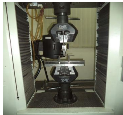
Fig. 5 Three point bending test
