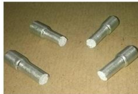
Figure 8 Tensile Test Specimens
