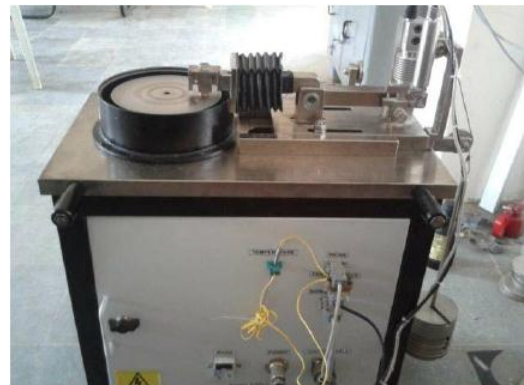
Figure 4 Pin- on- disc wear test rig
