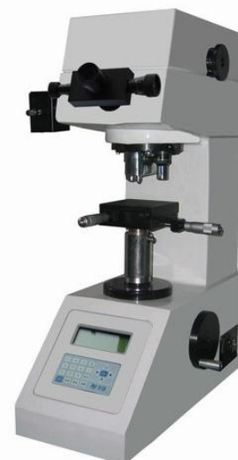
Figure 5 Vicker's Hardness Testing Machine
