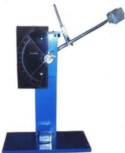
Figure 10 Izod Impact pendulum machine
