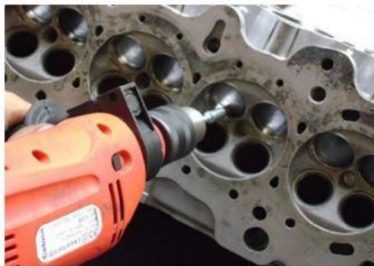
Figure Valve lapping using a power tool
