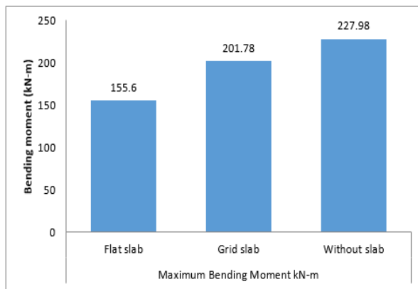
Fig 4: Max. Bending Moment
