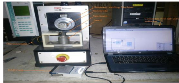
Experimental set up with temperature measurement attachment
