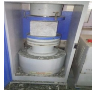
Figure 4(a): testing of cubes in compressive testing machine
