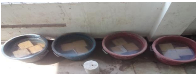
Figure 3(b): showing cubes in curing
