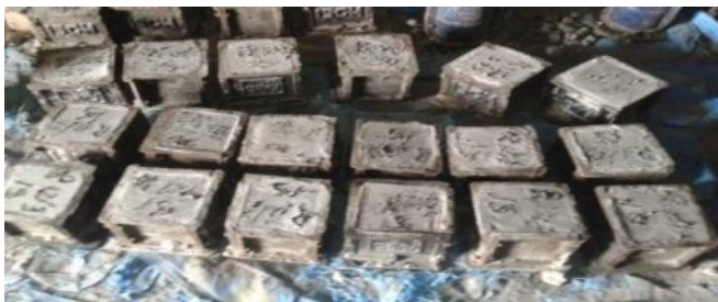
Figure 3(a): showing cubes compacted with concrete
