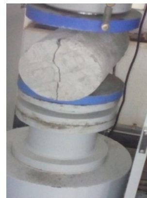
Figure 4(b): Testing of cylinders in compressive testing machine
