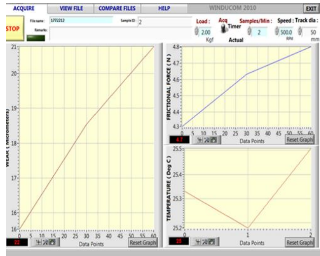
FIGURE 4: Wear graph- sample A at load 20kg
