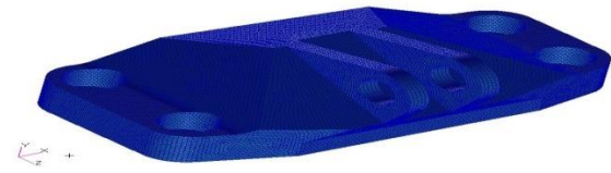
Original meshed model of engine bracket
