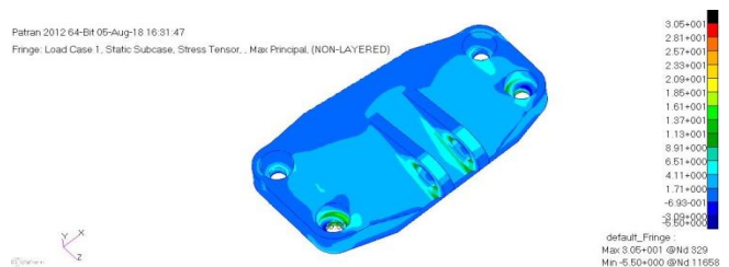
Max Principal Stress for vertical load
