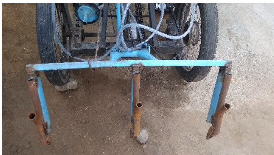
Fig. cultivator cum seed drill
