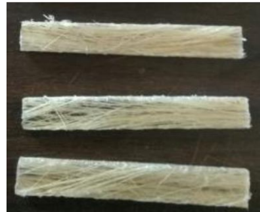
Fig.3.2 Test specimens for Impact Test
