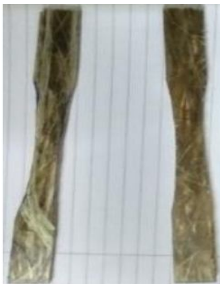
Fig.3.1. Test Specimens for Tensile and Compressive Test
