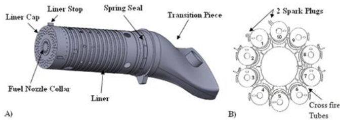
Fig. 3 (a) Schematic of the combustion chamber; (b) arrangement of the chambers on the rotor
