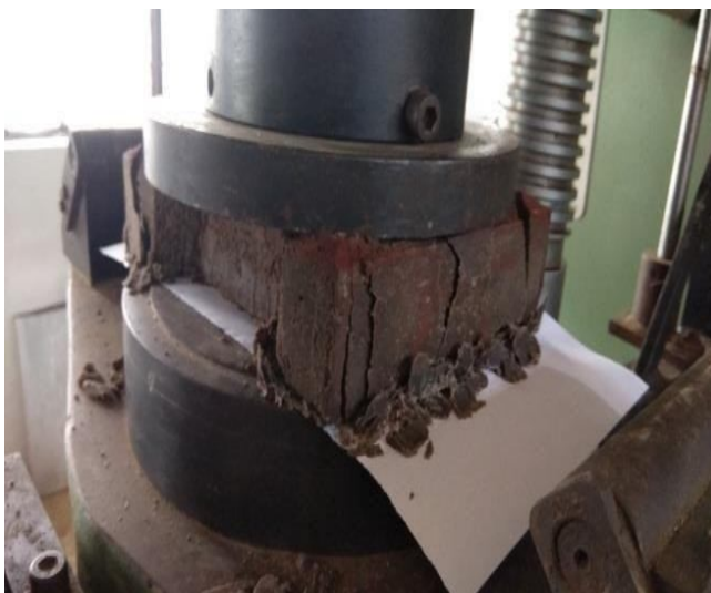
Fig 5.2: Compressive strength for plastic sand paver blocks
