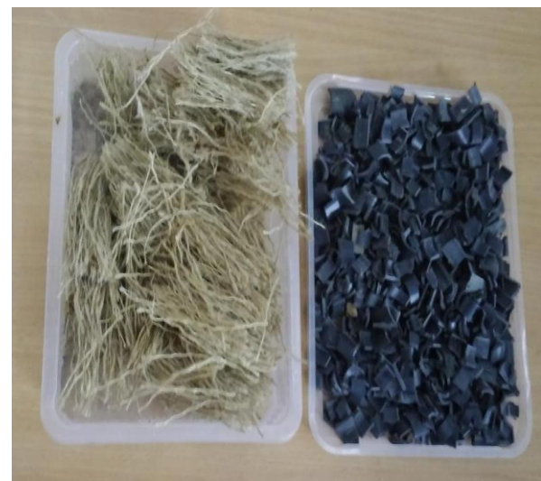
Fig. 2: Jute (Natural Fibre) with aspect ratio And Plastic Pipe Chip (Artificial Fibre)
