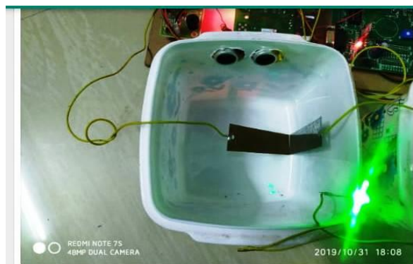
Fig5.2: Power Generation in Garbage Bin1, When Green LED as Indication of Power Generation
