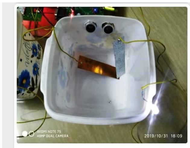
Fig5.3: Power Generation in Garbage Bin2, when white LED as Indication of Power Generation
