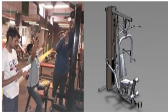
Figure 5: Proposed Design of Lat Pull Down Machine on Solidworks.
