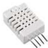
Fig.4.2: DHT22 Humidity Sensor
