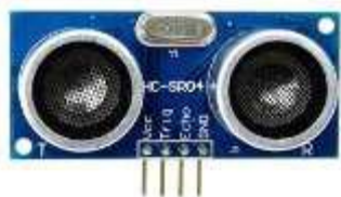
Fig. 4.1: HC-SR04 Ultrasonic Sensor
