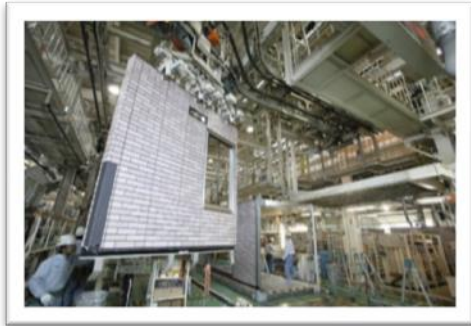
Fig. 1 The concept of Robotic Industrialization applied by the Japanese company Sekisui Heim to industrially personalize buildings on the assembly line (Image: courtesy of Sekisui Heim).
