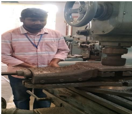
Figure 9. Face Milling Operation
