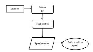
It is used to less fuel when it reaches public place. When fuel is less cant raise must down the gear so again apply break and move gear. By applying break he will come to the speed limited set by us. Complete process must not exceed 5 to 6 seconds. It must reduce vehicle speed not stop the vehicle.
